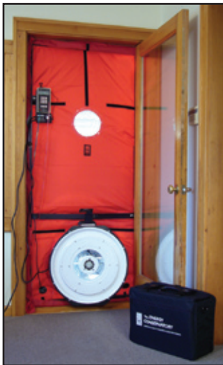
The Minneapolis Blower Door™ is used to measure the airtightness of buildings.
