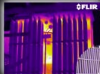
Plugged cooling fins on 13.8KV transformer
