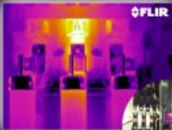
Connection problem on 200 Amp fused disconnect
