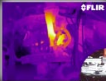
Overheating on water-cooled supply cable for robotic welder
