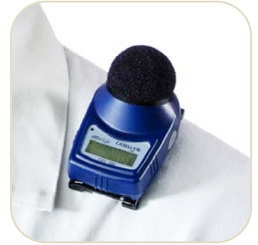
CEL-350 mounted on a shoulder using CEL-6351
